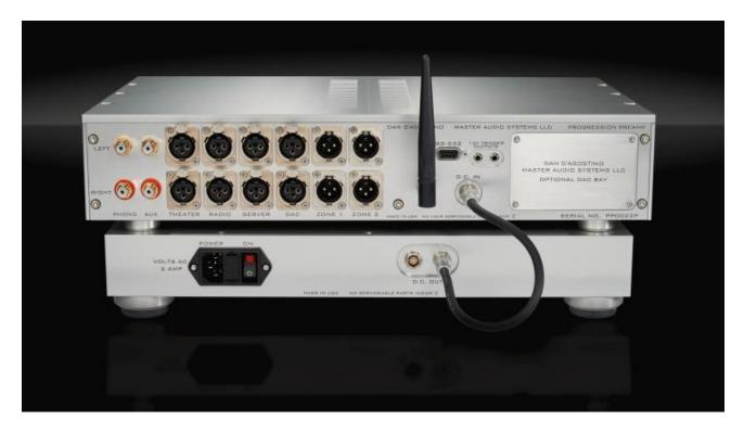
The top chassis has two analog audio boards, one for each channel. There are two pairs of singleended inputs, four pairs of balanced inputs, and two pairs of balanced outputs. Interestingly, one of the pairs of single ended-inputs is labeled "phono," but there is no phono stage. Maybe another hint at future plans?
